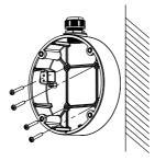
Figure 2-7 Secure the Junction Box on the Wall
