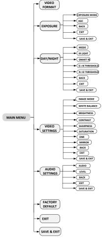
Figure 3-2 Main Menu Overview 5. Click the direction arrow to control the camera.
